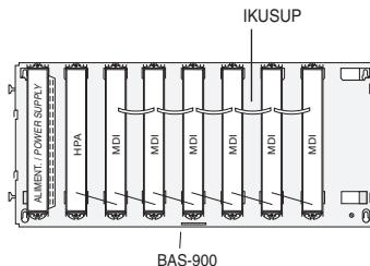
The pictures show two examples of module placement in MDI assemblies. The HPA amplifier must be placed at the end of the transmodulators' cascade. The power supply module/s must be always placed at the assembly's edges. If the NIT table must be adapted, the IKUSUP bus must be installed along the modules. The last transmodulator at the right end will carry out the control function.
